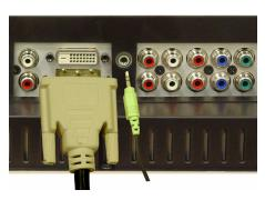
A digital signal that can support digital and convert analog to digital. DVI can be used for high resolution display and can support resolutions up to 1280 x 768.
